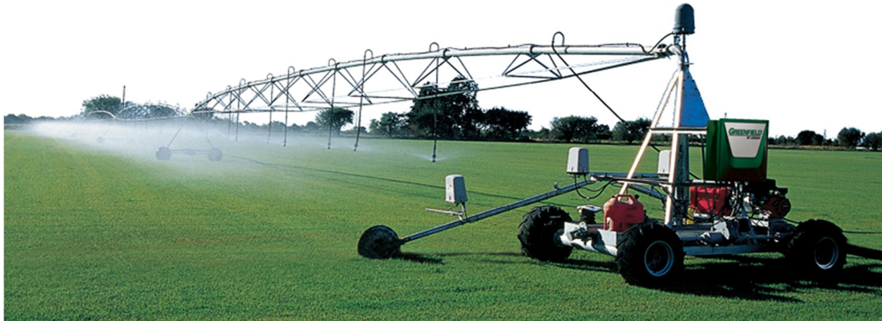
Figure 2-3b: Photo of a Lindsay Lateral move system (Photo from the Lindsay Greenfield ML400 Brochure)
